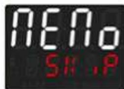
In order to save a parameter configuration in the memory card, connect it to micro-USB connector and power the instrument. If the memory has never been configured, the device starts normally, but if its data are considered valid, it is possible to view on the display AERo S...P. Press SET in order to start the product without uploading any data from the memory card. Configure, set the parameters and exit configuration. Now, the device saves the configuration just created also in the memory.
