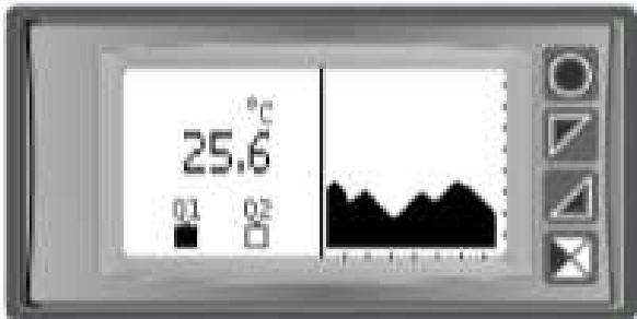
This page displays the process, the relays status and a graph representing the process trend.
