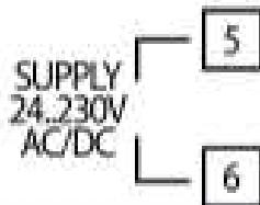
Switching supply with extended range 24...230 Vac/dc
