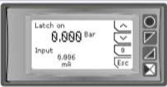
To use the LATCH ON function: enter configuration, select Setting on par. 8 Latch on and press "Sel" (STR551 shows the page in the picture).
