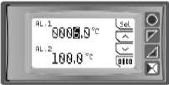
Press "Setpoint" to enter the thresholds modification.
