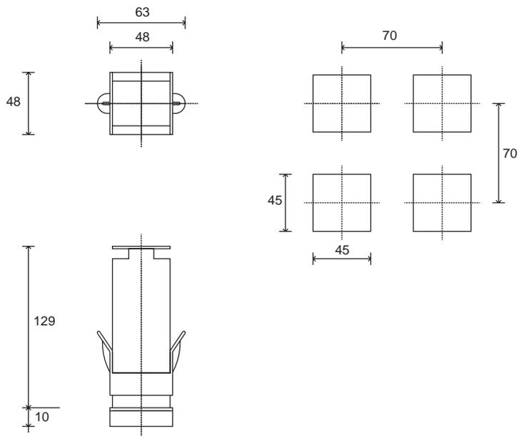
Dimensions: 48x48mm (1/16DIN), profondeur 129mm
